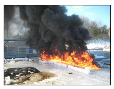
In image, burning of crude oil collected in a recovery trench. In foreground, a pit containing oil residue in broken ice is visible from previous burn. This is an accepted and extremely efficient method of mitigating oil spills in ice-infested waters.
